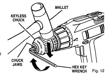
Open chuck jaws and remove hex key wrench. Remove the chuck screw by turning it in a clockwise direction. See Figure 13.
